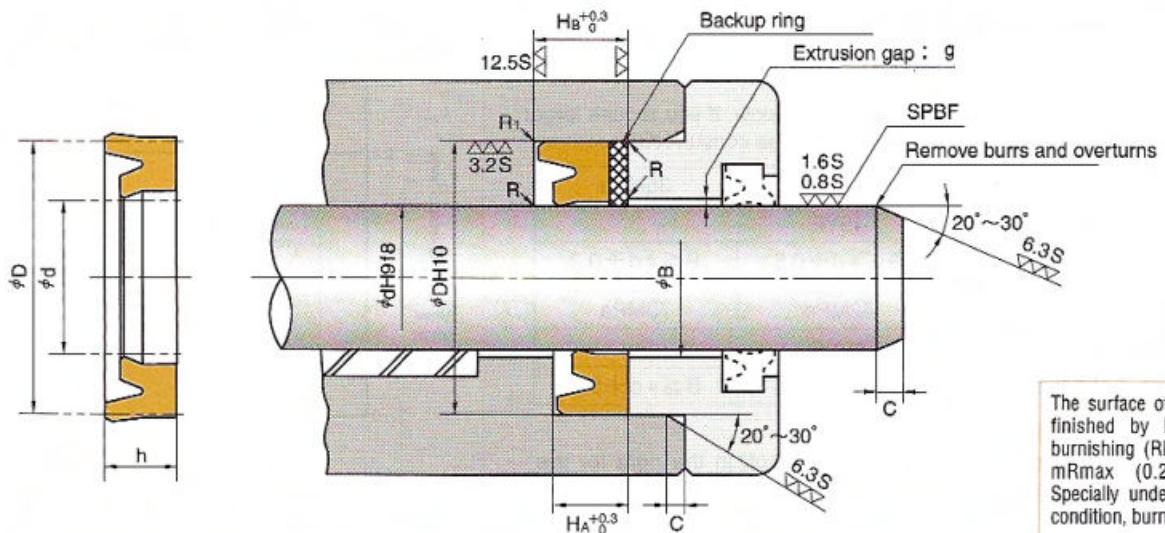
The surface of the rod should be finished by buffering (SPBF) or burnishing (RLB) to 0.8 to 1.6  $\mu\text{mR}_{\text{max}}$  (0.2 to 0.4  $\mu\text{mRa}$ ). Specially under severe lubricating condition, burnishing is required.
