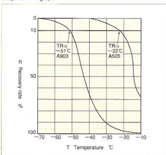
TR<sub>10</sub> values can indicate allowable low temperature service range of rubber material for packings. For allowable low temperature service range of specific types of packings, refer to page D-2 to 4.
