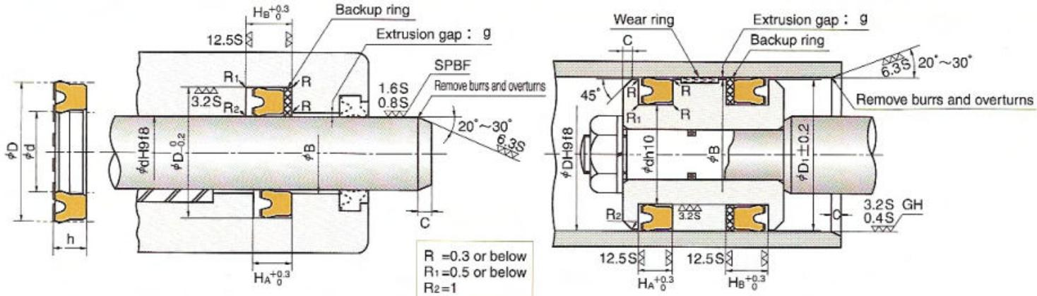
The surface of the rod should be finished by buffing (SPBF) or burnishing (RLB) to 0.8 to 1.6  $\mu\text{m}$  Rmax (0.2 to 0.4  $\mu\text{m}$  Ra). Specially under severe lubricating condition, burnishing is required.
