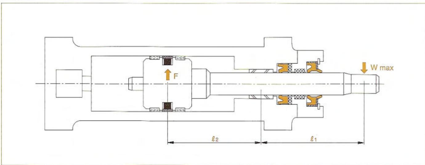
For example, if the calculation result of  $\phi 100\text{mm}$  diameter shows  $h_{\min} 17.5\text{mm}$ , use two GW0332PO (WR94  $\times$  100  $\times$  15) in dimension table on page F-134 or one GW0041P3 (WR94  $\times$  100  $\times$  25) in dimension table on page F-132. Sizes other than those in the dimension table are also available upon request. Please consult NOK. (Outer diameters up to  $\phi 800\text{mm}$  can be supplied.)
