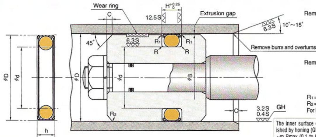
Remark 1) To determine  $\phi B$  dimension, please make the maximum extrusion gap (also refer page 26) 0.4mm or below considering the eccentricity of piston.
