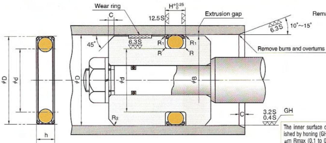
Remark 1) To determine  $\phi B$  dimension, please make the maximum extrusion gap (also refer page 26) 0.4mm or below considering the eccentricity of piston.
