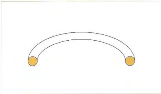
An O-ring (Fig. A-4) with an O-shaped profile is a typical squeeze packing. Significant pressure on the sealing surface is required to compress and deform the profile for sealing. For this reason, significant frictional resistance and high-sliding frictional heat is created resulting in a short life of the packing. To reduce sliding frictional resistance and frictional heat, the compression and deformation ratio of the O-ring should be decreased, which will, however, reduce the sealing ability.
