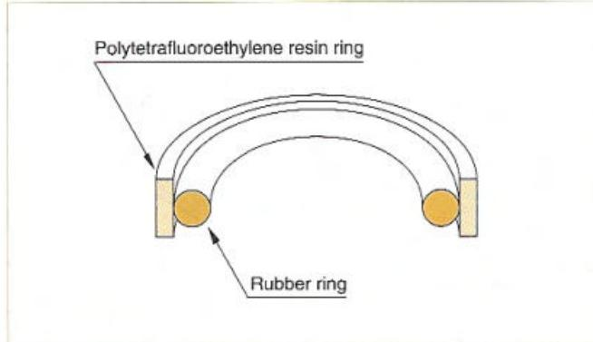
To decrease friction, a combined seal (called a slipper seal) has been developed with low-friction polytetra-fluoroethylene resin (PTFE) on the sliding surface (Fig. A-5).
