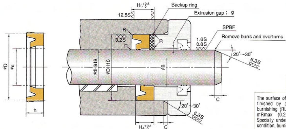
The surface of the rod should be finished by buffering (SPBF) or burnishing (RLB) to 0.8 to 1.6  $\mu$ mRmax (0.2 to 0.4  $\mu$ mRa). Specially under severe lubricating condition, burnishing is required.
