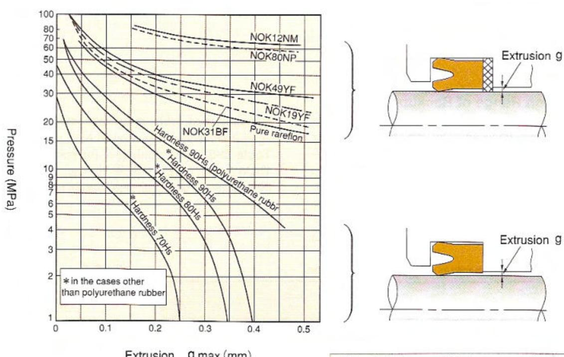
Note: Extrusion gap "g" is the amount of radius gap and calculated by a diameter clearance / 2.
