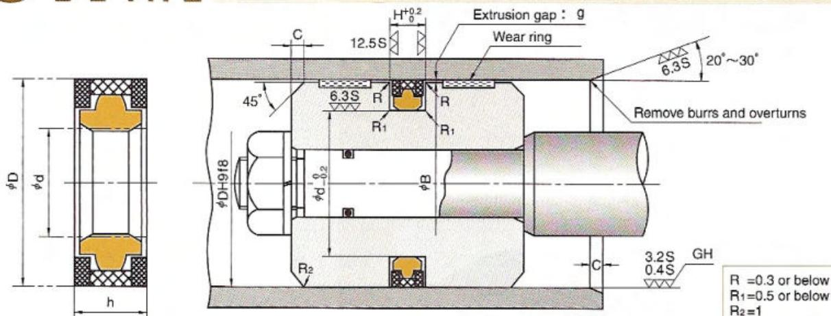
The inner surface of the cylinder tube should be finished by honing (GH) or burnishing (RLB) to 0.4 to 3.2  $\mu\text{m}$  Rmax (0.1 to 0.8  $\mu\text{m}$  Ra). Specially under severe lubricating condition, burnishing is required.
