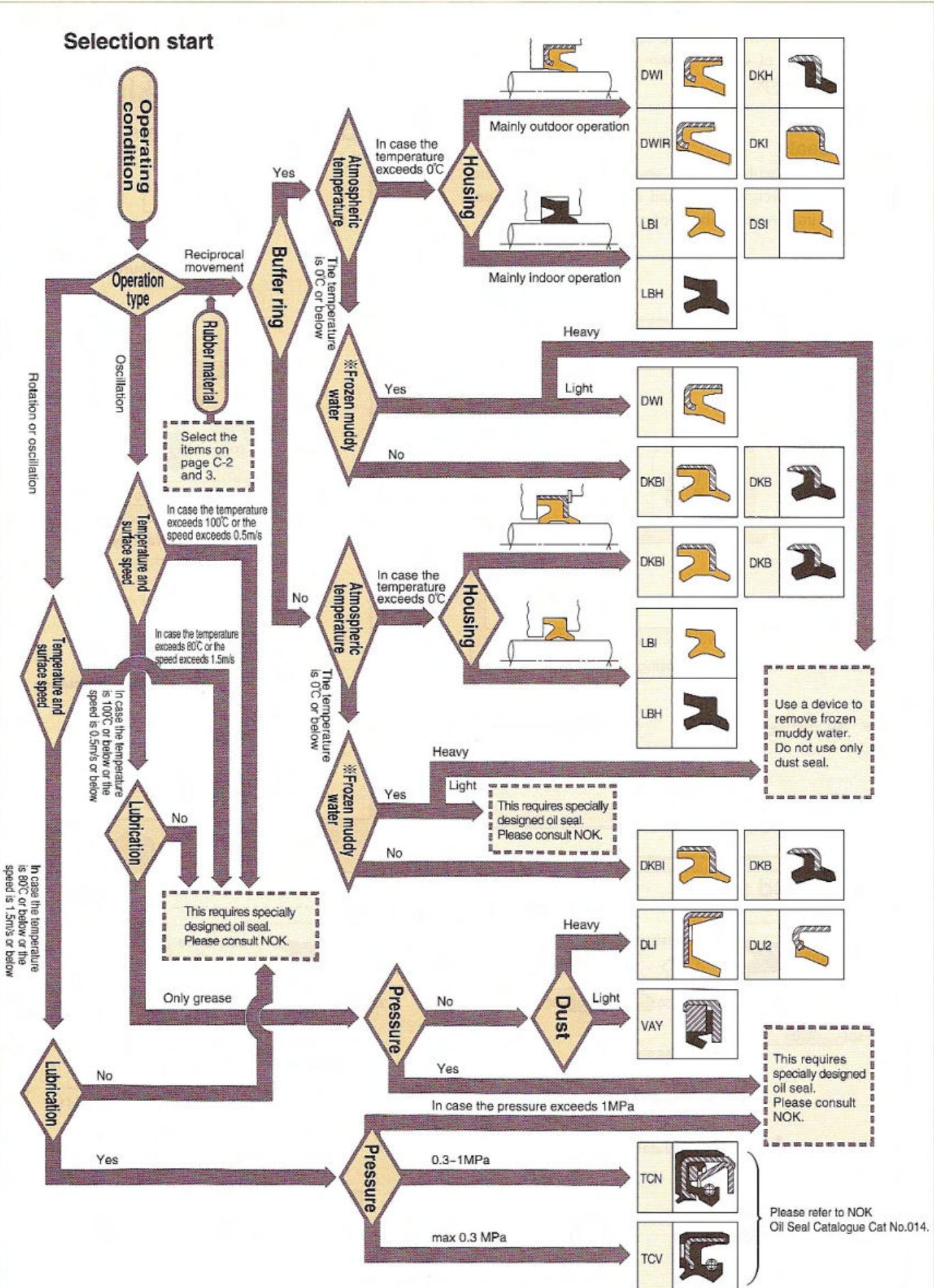
\* frozen muddy water : This is a condition where water on the rod surface has frozen. (It is the case that water is put on the rod during daytime operation and it has frozen in night time low temperature.)
