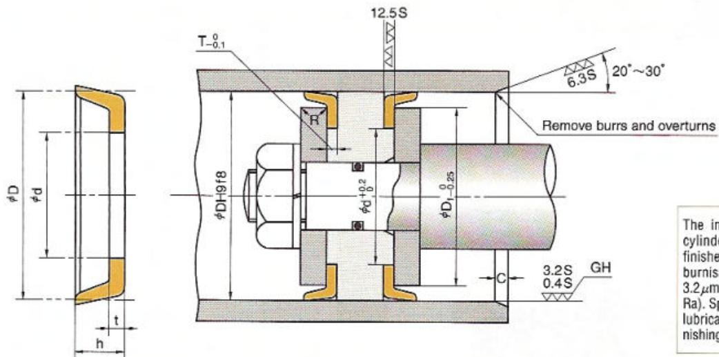
The inner surface of the cylinder tube should be finished by honing (GH) or burnishing (RLB) to 0.4 to 3.2  $\mu\text{m}$  Rmax (0.1 to 0.8  $\mu\text{m}$  Ra). Specially under severe lubricating condition, burnishing is required.
