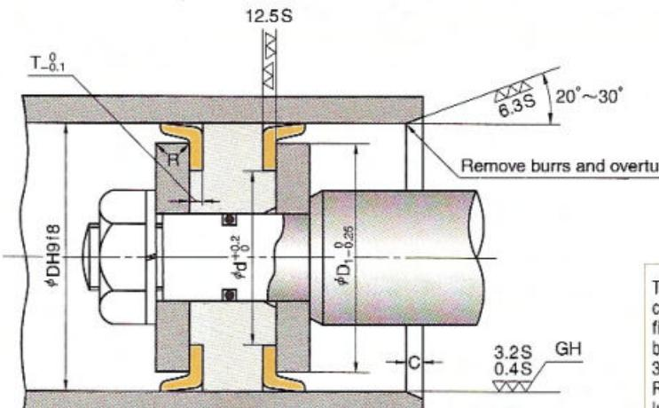
The inner surface of the cylinder tube should be finished by honing (GH) or burnishing (RLB) to 0.4 to 3.2  $\mu\text{m}$  Rmax (0.1 to 0.8  $\mu\text{m}$  Ra). Specially under severe lubricating condition, burnishing is required.
