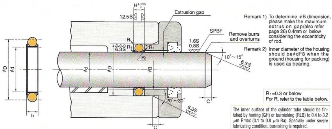
The inner surface of the cylinder tube should be finished by honing (GH) or burnishing (RLB) to 0.4 to 3.2  $\mu m$  Rmax (0.1 to 0.8  $\mu m$  Ra). Specially under severe lubricating condition, burnishing is required.
