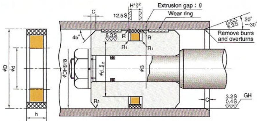
The inner surface of the cylinder tube should be finished by honing (GH) or burnishing (RLB) to 0.4 to 3.2  $\mu\text{m}$  Rmax (0.1 to 0.8  $\mu\text{m}$  Ra). Specially under severe lubricating condition, burnishing is required.
